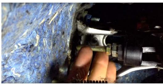
4. Underneath the vehicle, make sure that the slave cylinder can be depressed by hand and that it pushes fluid back up to the master cylinder. This ensures that the bearing does not hold on to the clutch diaphragm as the clutch wears.
