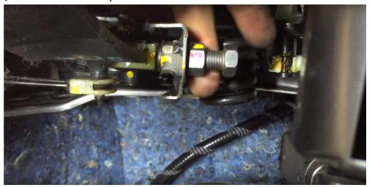
3. Adjust the pushrod from the master cylinder to the pedal by undoing the locking nut and rotating the pushrod. This must retain freeplay and should be able to be wriggled by hand. This is to ensure that there is no excess pressure on the master cylinder. Failure to do so could lead to premature clutch slipping. Tighten the locking nut to ensure that the pushrod does not adjust as the clutch is operated.
